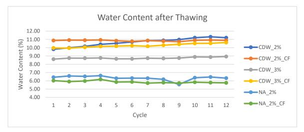
Figure 5- Water content of the specimens after the thaw situation
