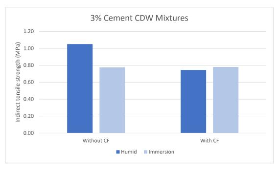
Figure 8 - Average results of the indirect tensile test for the 3% Cement CDW Mixtures
