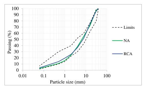
Figure 1 - Grain size distribution of recycled and natural aggregates (adapted from Crucho, 2021)
