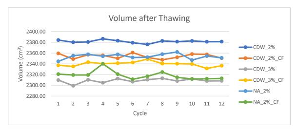
Figure 3 - Volume of the specimens after the thaw situation
