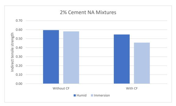
Figure 9 - Average results of the indirect tensile test for the 2% Cement NA Mixtures
