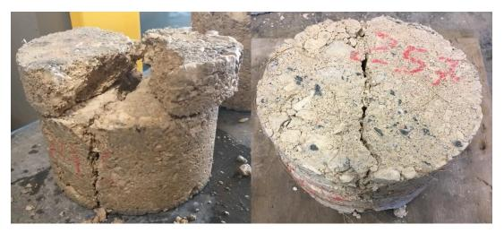
Figure 10 - Comparison between the final state of specimens without CF (left) and with CF (right)
