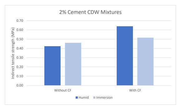
Figure 7 - Average results of the indirect tensile test for the 2% Cement CDW Mixtures
