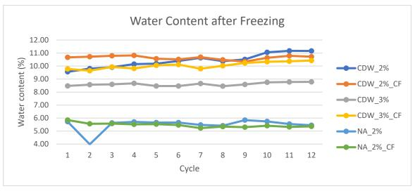
Figure 4- Water content of the specimens after the freeze situation
