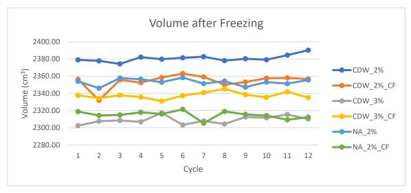
Figure 2 - Volume of the specimens after the freeze situation
